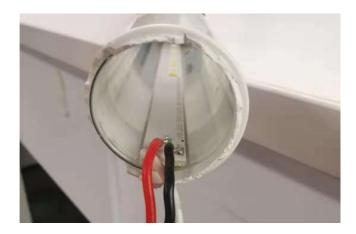
68. For example, the L13T8BY5041K has a diffusion film that is disposed on the glass tube to diffuse light emitted from the LEDs.
