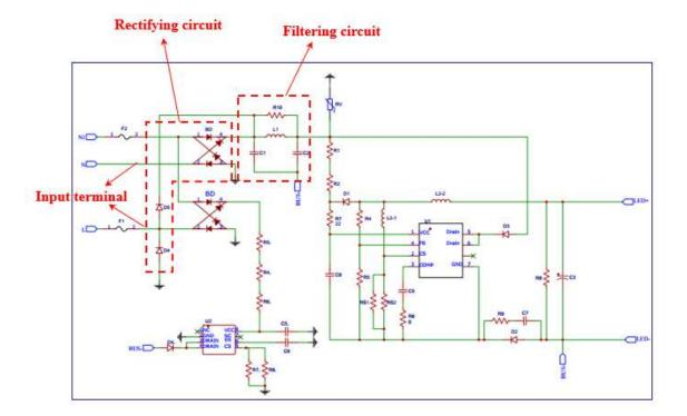
141. The electronic components on the printed circuit board further comprise a resistor which is positioned closest to the end wall of a first end cap and connects to one of the input terminals of the rectifying circuit.
