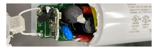
88. The 12.5W LED T8 UNIV 5000K 48" (3000705) has an installation detection circuit, *e.g.*, the CHP6061-MV1.0 with the DIO8270 Intelligent Power Protection Switch and associated circuitry. The CHP6061-MV1.0 with the DIO8270 receive an external driving signal.
