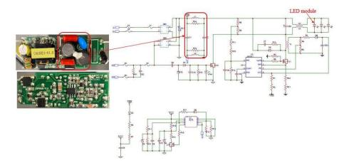
106. The tube lamp further comprises an LED module which includes LEDs for emitting light, and is configured to be driven either by the rectified signal or by the filtered signal:
