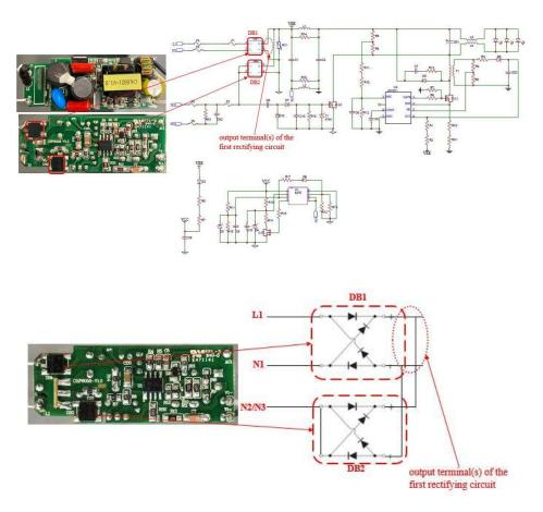
105. The tube lamp further comprises a filtering circuit coupled to the two rectifying circuits and an LED module for filtering the rectified signal to produce a filtered signal:
