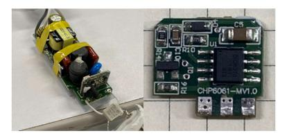
125. The CHP6061-MV1.0 has two devices connected in series, *e.g.*, R7 and C5, between an output terminal of the first rectifying circuit and ground. R7 and C5 provide a sampled signal on the node between them depending on the property of the rectified signal (VEE).
