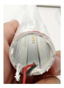
44. The connecting region includes at least two soldering pads for electrically connecting the power supply and "+" and "-" recognizing marks:
