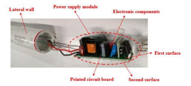
140. The electronic components on the printed circuit board include a rectifying circuit having at least two input terminals and configured to rectify a signal received from the at least two input terminals, and a filtering circuit electronically connected to the rectifying circuit:
