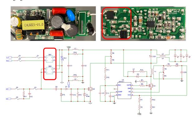
122. The 12.5W LED T8 UNIV 5000K 48" (3000705) has an LED module comprising LEDs for emitting light that are configured to be driven based on the rectified signal.
