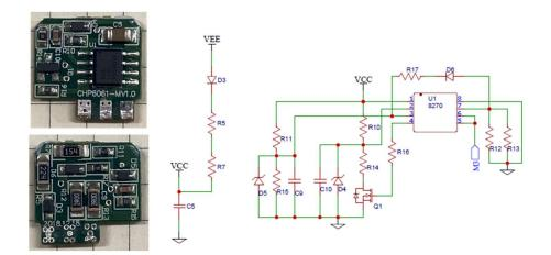
126. The DIO8270 provides a conduction path through the N-Type MOSFET in the DIO8270 between pins 5 and 7, causing the rectified signal to be used by the driving circuit to drive the LED module and emit light, when the sampled signal (VCC) is higher than a determined level.
